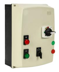
WEG Electric ESWE series combination Type-E motor starter, 38A, 3-pole, 208–240 VAC (60Hz)/180-208 VAC (50Hz) coil voltage, bimetallic, 25.0–32.0A adjustable, 416A instantaneous trip rating, NEMA 4/4X.
