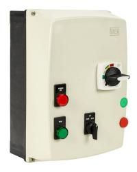
WEG Electric ESWE series combination Type-E motor starter, 25A, 3-pole, 120 VAC (50/60Hz) coil voltage, bi-metallic, 16.0–20.0A adjustable, 260A instantaneous trip rating, NEMA 4/4X.
