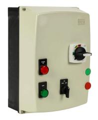
WEG Electric ESWE series combination Type-E motor starter, 18A, 3-pole, 480 VAC (50/60Hz) coil voltage, bi-metallic, 10.0–16.0A adjustable, 208A instantaneous trip rating, NEMA 4/4X.
