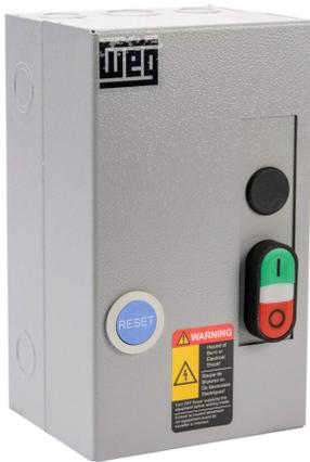
WEG Electric ESW series manual motor starter, pushbutton, 9A, 3-pole, 480 VAC (50/60Hz) coil voltage, thermal overload, 0.8-1.2A adjustable, NEMA 1.
