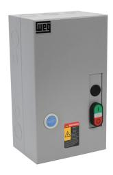
WEG Electric ESW series manual motor starter, pushbutton, 80A, 3-pole, 480 VAC (50/60Hz) coil voltage, thermal overload, 63.0-80.0A adjustable, NEMA 1.
