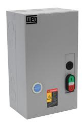
WEG Electric ESW series manual motor starter, pushbutton, 80A, 3-pole, 480 VAC (50/60Hz) coil voltage, thermal overload, 57.0-70.0A adjustable, NEMA 1.
