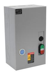
WEG Electric ESW series manual motor starter, pushbutton, 80A, 3-pole, 120 VAC (50/60Hz) coil voltage, thermal overload, 63.0-80.0A adjustable, NEMA 1.
