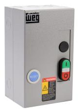
WEG Electric ESW series manual motor starter, pushbutton, 38A, 3-pole, 480 VAC (50/60Hz) coil voltage, thermal overload, 32.0-40.0A adjustable, NEMA 1.
