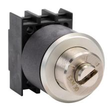
Schmersal selector switch, IP65, 30mm, 3-position, maintained, key removable right position, operator only, plastic base, metal bezel, Operator: black, key-operated, 36mm, round, metal. Requires contact blocks.
