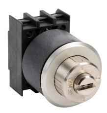
Schmersal selector switch, IP65, 30mm, 3-position, maintained, key removable left, right and center position, operator only, plastic base, metal bezel, Operator: black, key-operated, 36mm, round, metal. Requires contact blocks.
