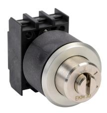
Schmersal selector switch, IP65, 30mm, 3-position, maintained, key removable left position, operator only, plastic base, metal bezel, Operator: black, key-operated, 36mm, round, metal. Requires contact blocks.
