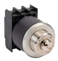
Schmersal selector switch, IP65, 30mm, 2-position, maintained, key removable left position, operator only, plastic base, metal bezel, Operator: black, key-operated, 36mm, round, metal. Requires contact blocks.
