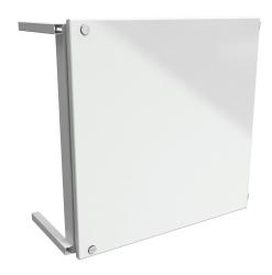
Hammond swing panel, carbon steel, RAL 9003 white, powder coat finish. For use with 24x24 (HxW) EN4SD2424xxx & ST2424xxx Eclipse series enclosures.
