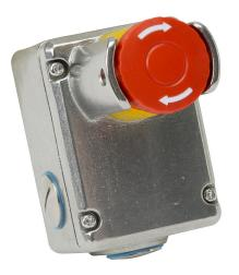
IDEM emergency stop control station, 316 stainless steel, single pushbutton, mushroom, red, twist-to-release, guarded, (4) N.C. contact(s).
