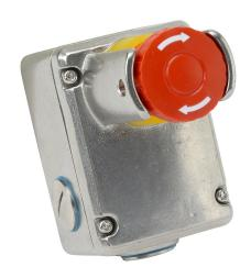
IDEM emergency stop control station, 316 stainless steel, single pushbutton, mushroom, red, twist-to-release, guarded, (2) N.O./ (2) N.C. contact(s).
