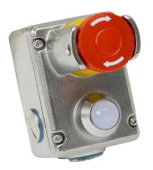
IDEM emergency stop control station, 316 stainless steel, single pushbutton, mushroom, red, 110 VAC LED, red/green, twist-to-release, guarded and padlockable, (1) N.O./(3) N.C. contact(s).
