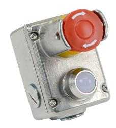
IDEM emergency stop control station, 316 stainless steel, single pushbutton, mushroom, red, 24 VDC LED, red/green, twist-to-release, guarded and padlockable, (1) N.O./(3) N.C. contact(s).
