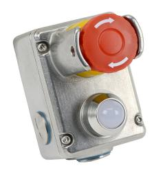
IDEM emergency stop control station, 316 stainless steel, single pushbutton, mushroom, red, 110 VAC LED, red/green, twist-to-release, guarded and padlockable, (2) N.O./(2) N.C. contact(s).
