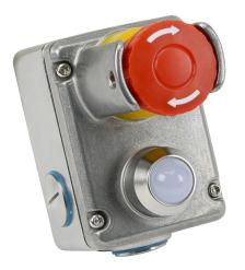
IDEM emergency stop control station, 316 stainless steel, single pushbutton, mushroom, red, 24 VDC LED, red/green, twist-to-release, guarded and padlockable, (2) N.O./(2) N.C. contact(s).
