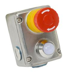
IDEM emergency stop control station, 316 stainless steel, single pushbutton, mushroom, red, 24 VDC LED, red/green, twist-to-release, (1) N.O./(3) N.C. contact(s).
