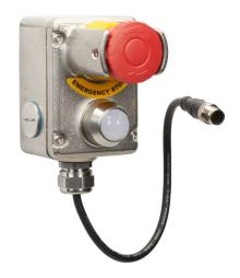
IDEM Z-Range emergency stop control station, 316 stainless steel, single pushbutton, mushroom, red, 24 VDC LED, red/green, twist-to-release, guarded, (2) OSSD safety output(s), 8-pin M12 quick-disconnect.
