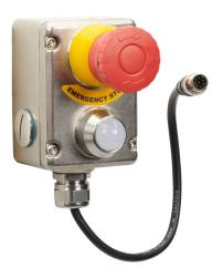
IDEM Z-Range emergency stop control station, 316 stainless steel, single pushbutton, mushroom, red, 24 VDC LED, red/green, twist-to-release, (2) OSSD safety output(s), 8-pin M12 quickdisconnect.
