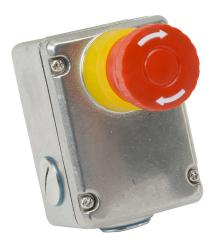
IDEM emergency stop control station, 316 stainless steel, single pushbutton, mushroom, red, twist-to-release, (1) N.O./(3) N.C. contact(s).
