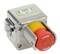
IDEM emergency stop control station, 316 stainless steel, single pushbutton, mushroom, red, twist-to-release, guarded and padlockable, (3) N.C. contact(s).
