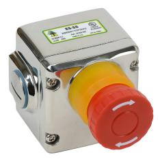
IDEM emergency stop control station, 316 stainless steel, single pushbutton, mushroom, red, twist-to-release, (3) N.C. contact(s).
