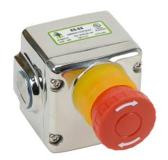
IDEM emergency stop control station, 316 stainless steel, single pushbutton, mushroom, red, twist-to-release, (1) N.O./(2) N.C. contact(s).
