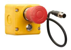
IDEM Z-Range emergency stop control station, plastic, single pushbutton, mushroom, red, 24 VDC LED, red/green, twist-to-release, (2) OSSD safety output(s), 8-pin M12 quick-disconnect, right exit.
