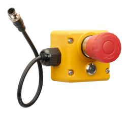
IDEM Z-Range emergency stop control station, plastic, single pushbutton, mushroom, red, 24 VDC LED, red/green, twist-to-release, (2) OSSD safety output(s), 8-pin M12 quick-disconnect, left exit.
