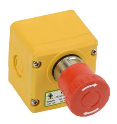
IDEM emergency stop control station, plastic, single pushbutton, mushroom, red, twist-to-release, (1) N.O./(2) N.C. contact(s).
