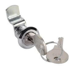
Hammond enclosure latch, replacement, keylocking, 1/4-turn semi-flush, 1-point, die-cast zinc, chrome finish. For use with Eclipse series swing-out panels. (2) keys included.
