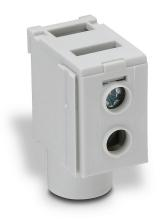
Edison direct feed wiring lug, 115A, 1000 VAC/VDC, 1 openings, #14-1 AWG copper only. For use with EB1P or EB3P series busbars.
