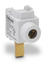
Edison box type wiring lug, 115A, 1000 VAC/VDC, 1 openings, #10 AWG-1/0 copper only. Package of 10. For use with EB1P series busbars.
