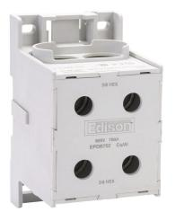
Edison enclosed power distribution block, finger-safe, 760A, 1-pole, line side: 2 openings accept 500 MCM to 6 AWG, load side: 2 openings accept 500 MCM to 6 AWG, panel mount, UL 1953 listed.
