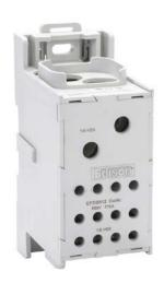
Edison enclosed power distribution block, 570A, 1-pole, line side: 2 openings accept 300 MCM to 4 AWG, load side: 12 openings accept 4AWG to 14 AWG, DIN rail mount, UL 1953 listed.
