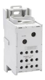
Edison enclosed power distribution block, finger-safe, 570A, 1-pole, line side: 2 openings accept 300 MCM to 4 AWG, load side: 12 openings accept 4AWG to 14 AWG, DIN rail mount, UL 1953 listed.
