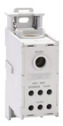
Edison enclosed power distribution block, 380A, 1-pole, line side: 1 opening accepts 500 MCM to 6 AWG, load side: 6 openings accept 2 AWG to 14 AWG, panel mount, UL 1953 listed.
