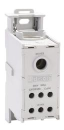
Edison enclosed power distribution block, finger-safe, 380A, 1-pole, line side: 1 opening accepts 500 MCM to 6 AWG, load side: 6 openings accept 2 AWG to 14 AWG, panel mount, UL 1953 listed.
