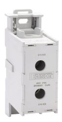
Edison enclosed power distribution block, 310A, 1-pole, line side: 1 opening accepts 350 MCM to 6 AWG, load side: 1 opening accepts 350 MCM to 8 AWG, DIN rail mount, UL 1953 listed.
