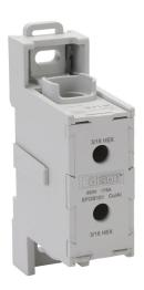
Edison enclosed power distribution block, 175A, 1-pole, line side: 1 opening accepts 2/0 AWG to 8 AWG, load side: 1 opening accepts 2/0 AWG to 8 AWG, DIN rail mount, UL 1953 listed.
