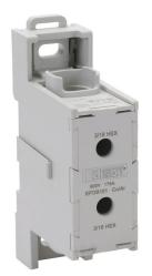
Edison enclosed power distribution block, finger-safe, 175A, 1-pole, line side: 1 opening accepts 2/0 AWG to 8 AWG, load side: 1 opening accepts 2/0 AWG to 8 AWG, DIN rail mount, UL 1953 listed.
