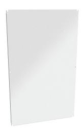
Hammond subpanel, carbon steel, RAL 9003 white, powder coat finish. For use with 48x30 (HxW) EN4SD4830xxx Eclipse series enclosures.
