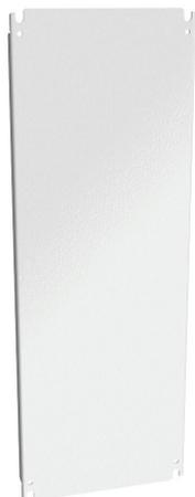
Hammond subpanel, carbon steel, RAL 9003 white, powder coat finish. For use with 30x12 (HxW) EN4SD30128xx Eclipse series enclosures.
