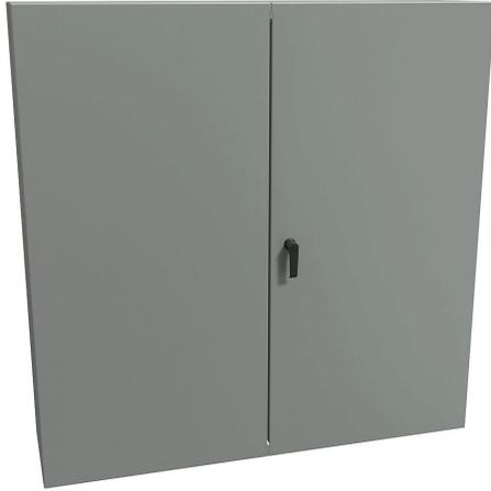
Hammond Eclipse series enclosure, NEMA 3R/12, 48 x 48 x 12in (HxWxD), wall mount, carbon steel, ANSI 61 gray, powder coat finish, double-door, 3-point keylocking handle.
