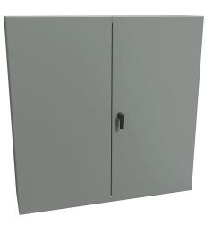
Hammond Eclipse series enclosure, NEMA 3R/12, 48 x 48 x 12in (HxWxD), wall mount, carbon steel, ANSI 61 gray, powder coat finish, double-door, 3-point keylocking handle.
