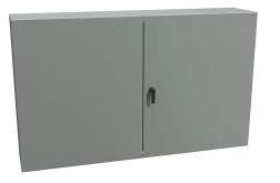
Hammond Eclipse series enclosure, NEMA 3R/12, 36 x 60 x 12in (HxWxD), wall mount, carbon steel, ANSI 61 gray, powder coat finish, double-door, 3-point keylocking handle.
