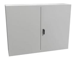
Hammond Eclipse series enclosure, NEMA 3R/12, 36 x 48 x 12in (HxWxD), wall mount, carbon steel, RAL 7035 light gray, powder coat finish, double-door, 3-point keylocking handle.
