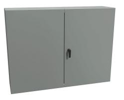
Hammond Eclipse series enclosure, NEMA 3R/12, 36 x 48 x 12in (HxWxD), wall mount, carbon steel, ANSI 61 gray, powder coat finish, double-door, 3-point keylocking handle.
