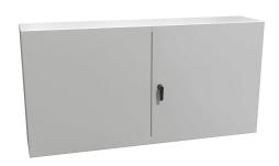
Hammond Eclipse series enclosure, NEMA 3R/12, 30 x 60 x 12in (HxWxD), wall mount, carbon steel, RAL 7035 light gray, powder coat finish, double-door, 3-point keylocking handle.
