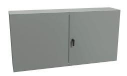
Hammond Eclipse series enclosure, NEMA 3R/12, 30 x 60 x 12in (HxWxD), wall mount, carbon steel, ANSI 61 gray, powder coat finish, double-door, 3-point keylocking handle.
