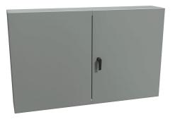
Hammond Eclipse series enclosure, NEMA 3R/12, 30 x 48 x 8in (HxWxD), wall mount, carbon steel, ANSI 61 gray, powder coat finish, double-door, 3-point keylocking handle.
