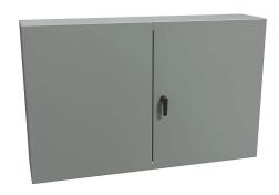
Hammond Eclipse series enclosure, NEMA 3R/12, 30 x 48 x 10in (HxWxD), wall mount, carbon steel, ANSI 61 gray, powder coat finish, double-door, 3-point keylocking handle.
