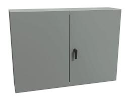
Hammond Eclipse series enclosure, NEMA 3R/12, 30 x 42 x 10in (HxWxD), wall mount, carbon steel, ANSI 61 gray, powder coat finish, double-door, 3-point keylocking handle.
