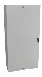
Hammond Eclipse series enclosure, NEMA 3R/4/12, 72 x 36 x 16in (HxWxD), wall mount, carbon steel, RAL 7035 light gray, powder coat finish, single-door, 3-point keylocking handle.
