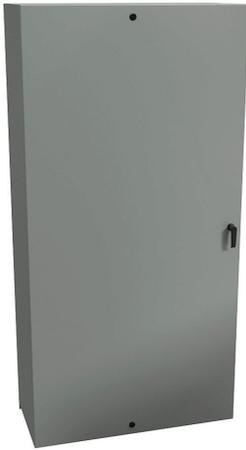
Hammond Eclipse series enclosure, NEMA 3R/4/12, 72 x 36 x 16in (HxWxD), wall mount, carbon steel, ANSI 61 gray, powder coat finish, single-door, 3-point keylocking handle.
